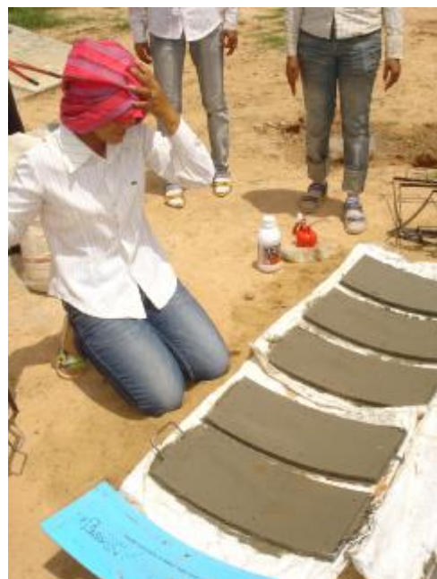
Figure 2 – Filling the cement brick moulds
